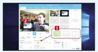
The tabs across the bottom provide tools for adjusting different elements of the video, though some are only available if you upgrade. For example, on the Image tab, you can select Picture in Picture mode 11 which overlays one of your cameras in a box over the other. 2
